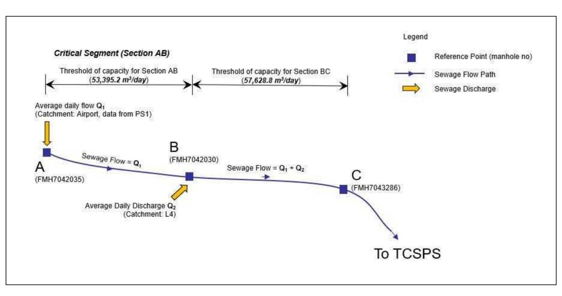
FIGURE 2.8 SCHEMATIC DIAGRAM FOR SEWERAGE SYSTEM FLOW MONITORING
